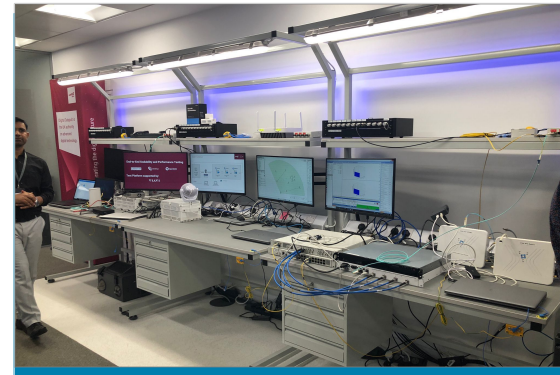
5G RAN including RIC tested under various interoperability conditions in Sonic Lab, London
