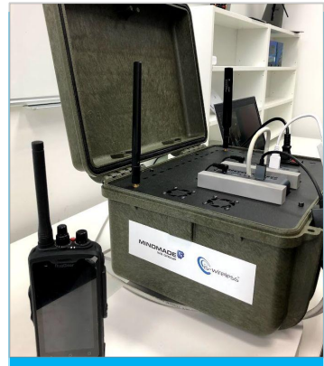
Complete 4G or 5G network in a box (RAN+Core) with MC applications (e.g., PTT)
