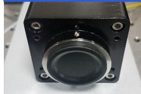
InGaAs Sensor 640 x 512 pixels (400 nm - 1700nm)
