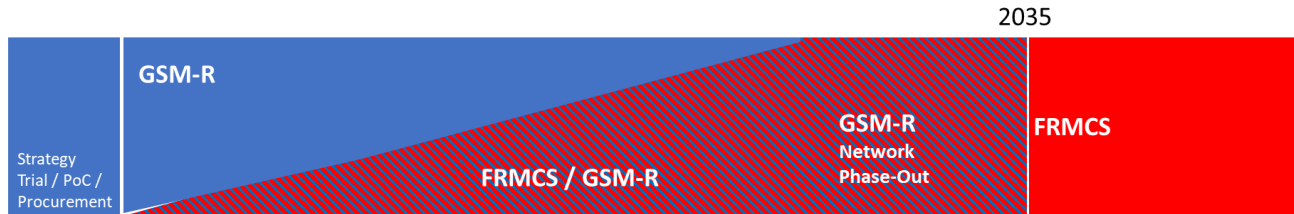
Figure 12: Indicative transition from GSM-R to FRMCS 5G SA and beyond.
