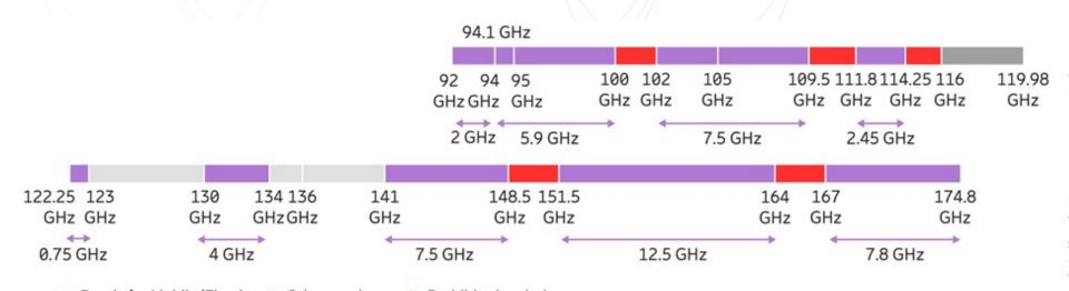
Figure 1. Frequency bands which are currently discussed for wide bandwidth 6G mobile communication (Source: https://www.ericsson.com/en/blog/2022/6/6g-spectrum-why-its-fundamental)
