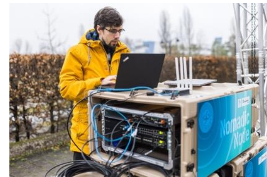
Mobile testbed: 5Genesis project, ALADIN, CampusOS 5G out of the box with our modular Nomadic Node
