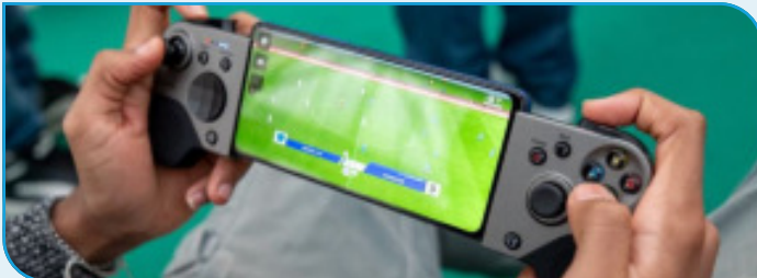
Figure 7.2: Handheld user kit including a portable low-latency telescopic controller and 5G smartphone.
